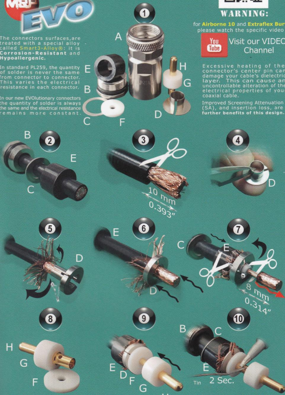
No more solder burrs on the pin which, being rounded, will enter smoothly.
